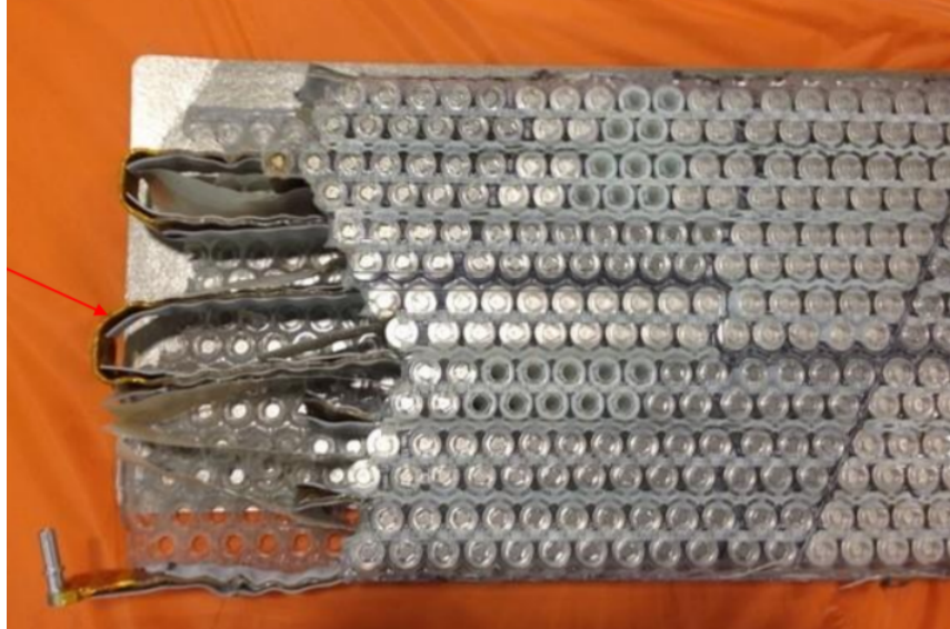
Figure 11:- Tesla's Model S Battery Module with Thermal Management System (Albright, 2018)
