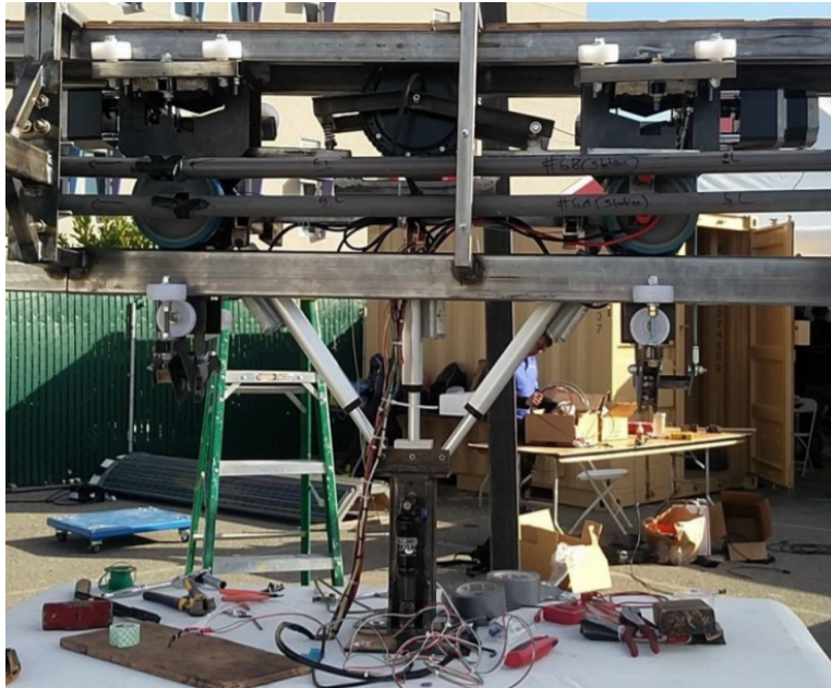
Figure 10:- SPARTAN Superway Bogie Assembly Class of 2016 (Acoba et al., 2016). Utilizing three shock absorbers to hold the cabin doubles as suspension.
