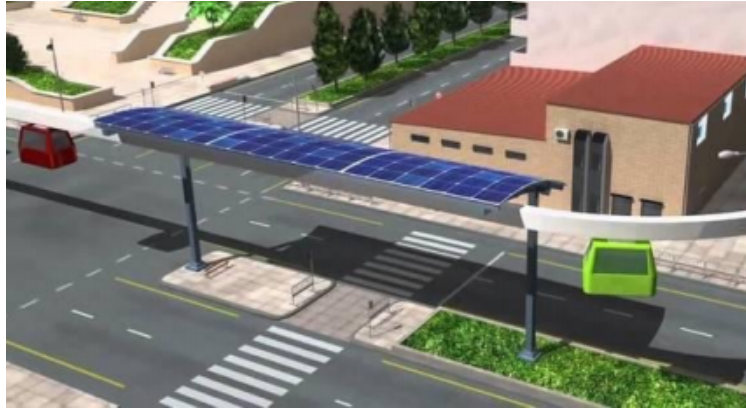
Figure 1:- Solar-powered automated transit (Hagstrom et al., 2017). Relatively small vehicles used on a slim guideway to provide non stop travel utilizing offline stations.
