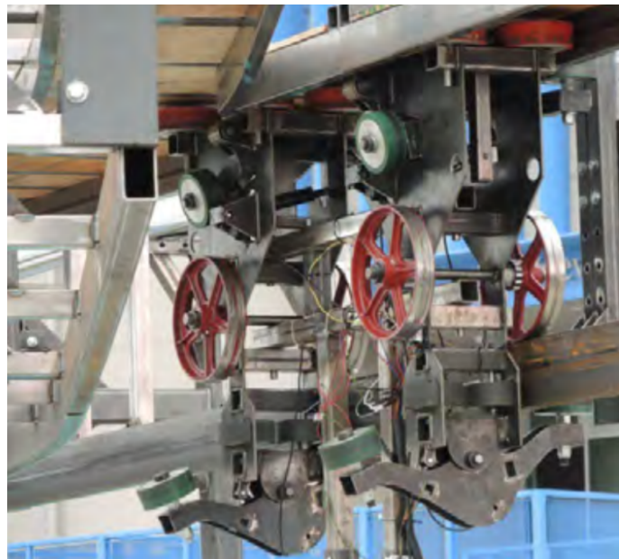
Figure 3:- Bogie with a steering mechanism on a guideway junction shown at Maker Faire 2015 (Furman, 2016).
