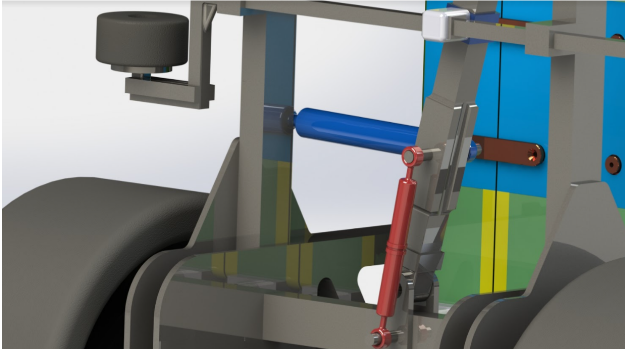
Figure 17:- Bogie switch mechanism is controlled using a hydraulic linear actuator and a stretched spring is used as a fail-safe.
