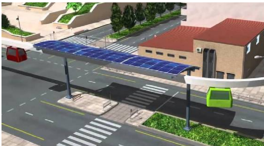
Figure 1. SPARTAN Superway Concept. Relatively small vehicles traverse a network of exclusive guideways and utilize off-line stations to provide on-demand, non-stop, origin-to-destination mobility. Suspending the ATN vehicle below the guideway makes the upper surface available for PV panels that can power the system.
