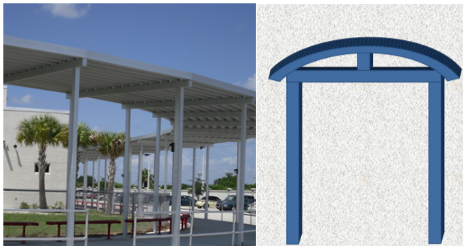
Figure 14. Profiles from Perfection Architectural Systems. A curved section of a flat canopy from Perfection Architectural Systems, LLC that could be used as a model to curve the Superway's canopy on the left and a curved understructure is shown on the right (Flat Canopy and Solar Framing, from (Perfection Architectural Systems, 2013)).
