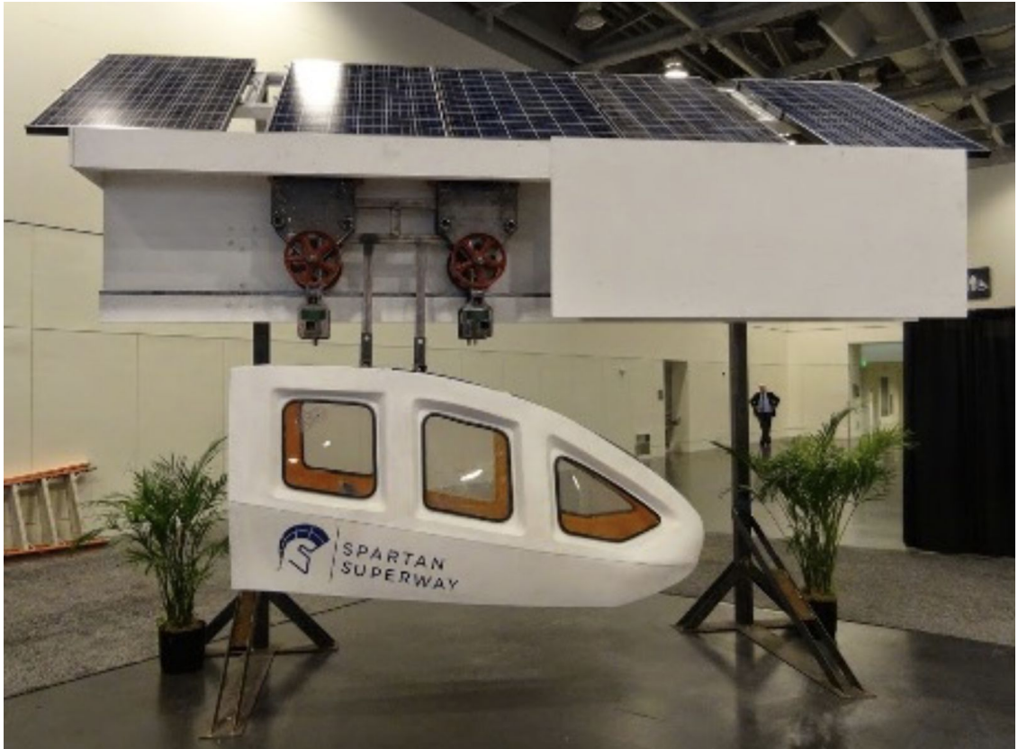
Figure 9: Spartan Superway with its clean energy source
