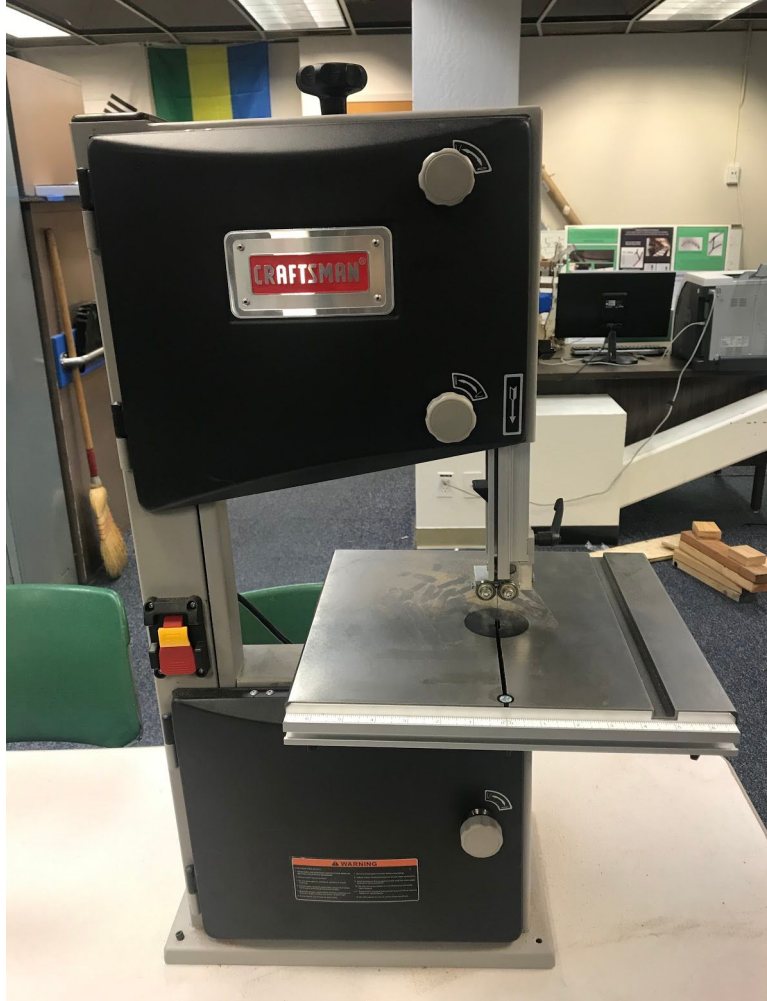
Figure 16: The device used to cut the track pieces when water jetting isn't available
