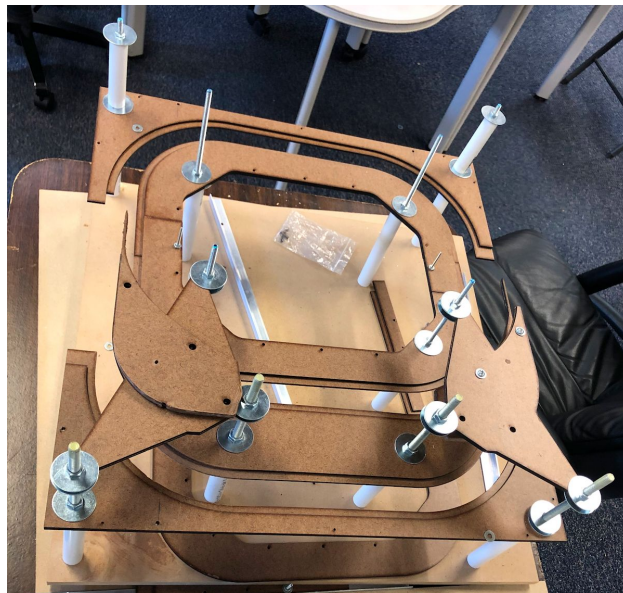
Figure 14. Bill James first prototype of mini-scale model using threaded studs.
