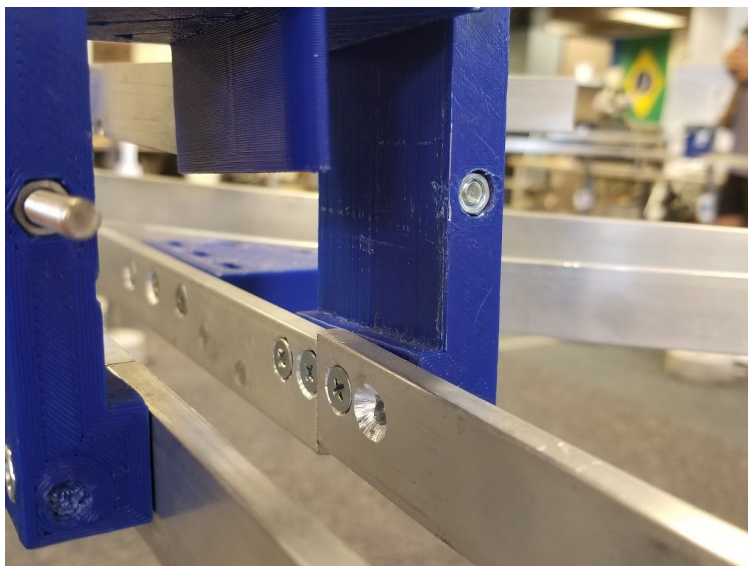
Figure 13. Connection between two tracks
