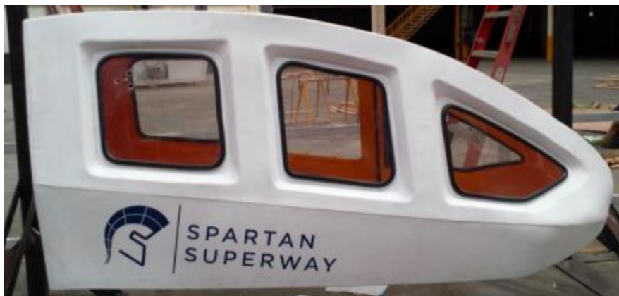
Figure 11. SPARTAN Superway Full-Scale Cabin
