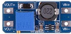
Figure 13. The boost converter increases voltage current at the cost of decreasing current; it was placed after the battery charger and before the Arduino and stepper motor driver board.
