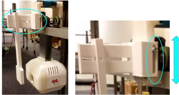
Figure 7. The T-shaped piece of the charging station has a cut-out slot for height adjustment.
