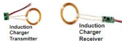
Figure 3. The induction module used was a 12V, 600 mA wireless charging module with a maximum charging distance of 0.787 inches.
