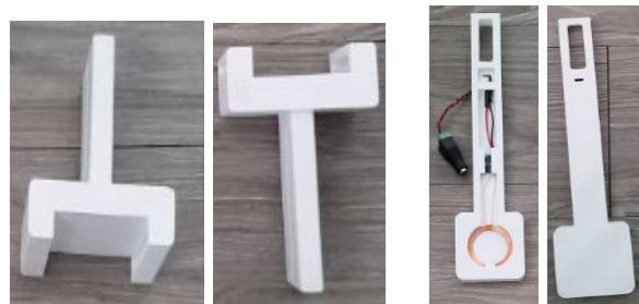
Figure 6. Two separate pieces constitute the induction charging hub: a T-shaped foundation piece and a spatula-shaped piece that slides onto the foundation piece and hangs from it.
