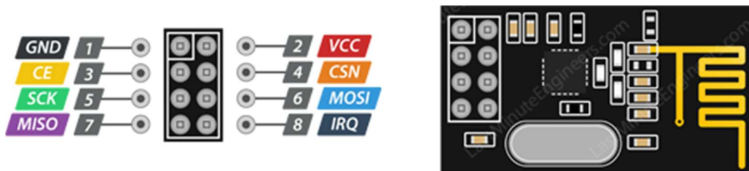
Figure 46: Pin Layout on the NRF24L01.
