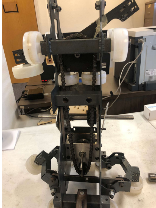
Figure 10: The new gears and roller chain mounted on the bogie.
