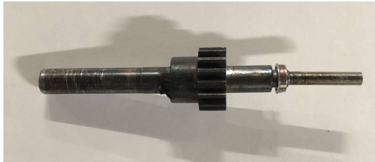
Figure 12: The old upper shaft with existing gear and bearings.
