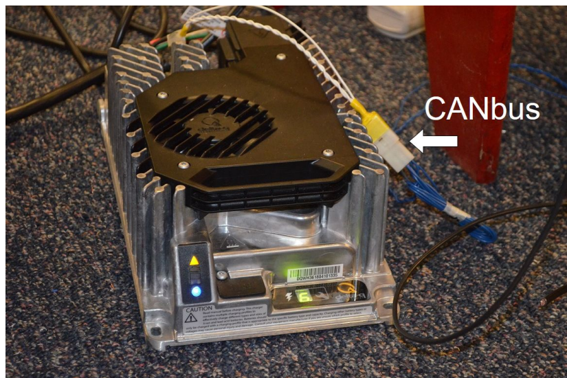
Figure 13: Delta-Q IC 1200W Charger and the CANbus communication quick plug-in port as the charger is not located on the bogie (off-board).
