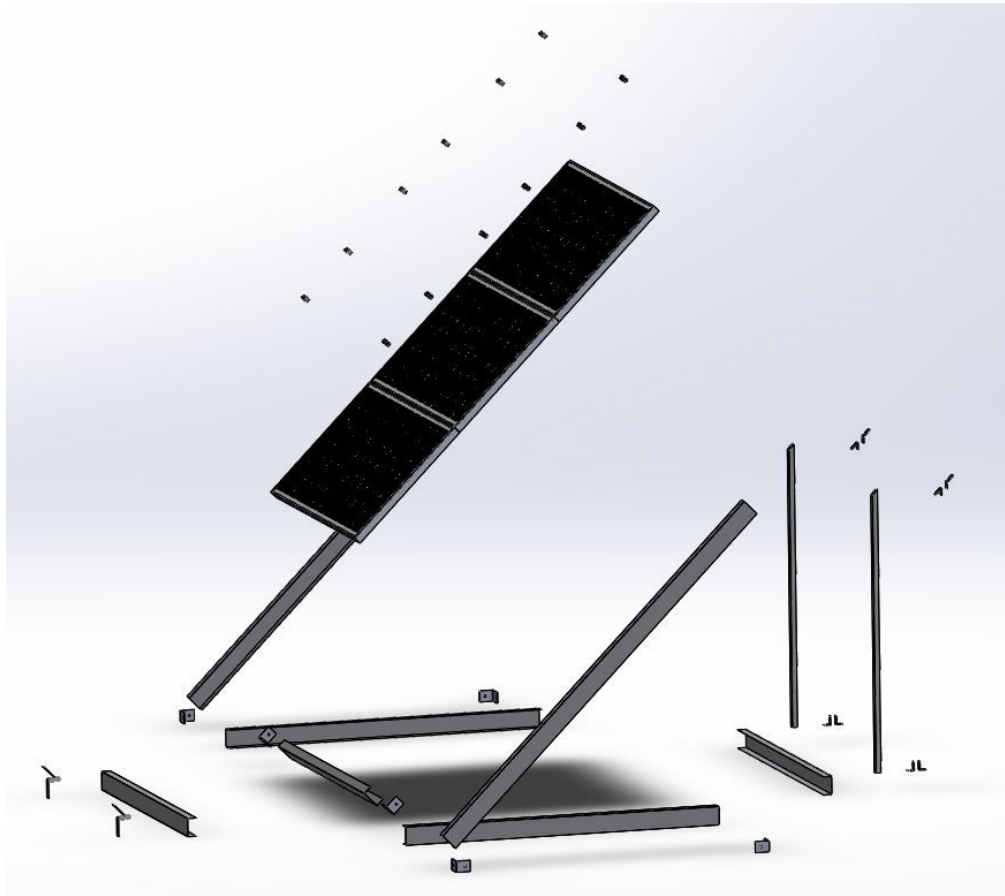
Figure 10. Exploded CAD view of the 3 panel solar array.
