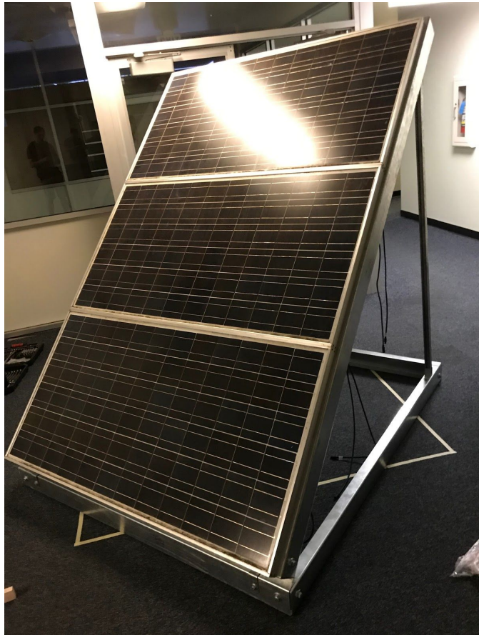
Figure 8. Constructed 3 panel solar array.
