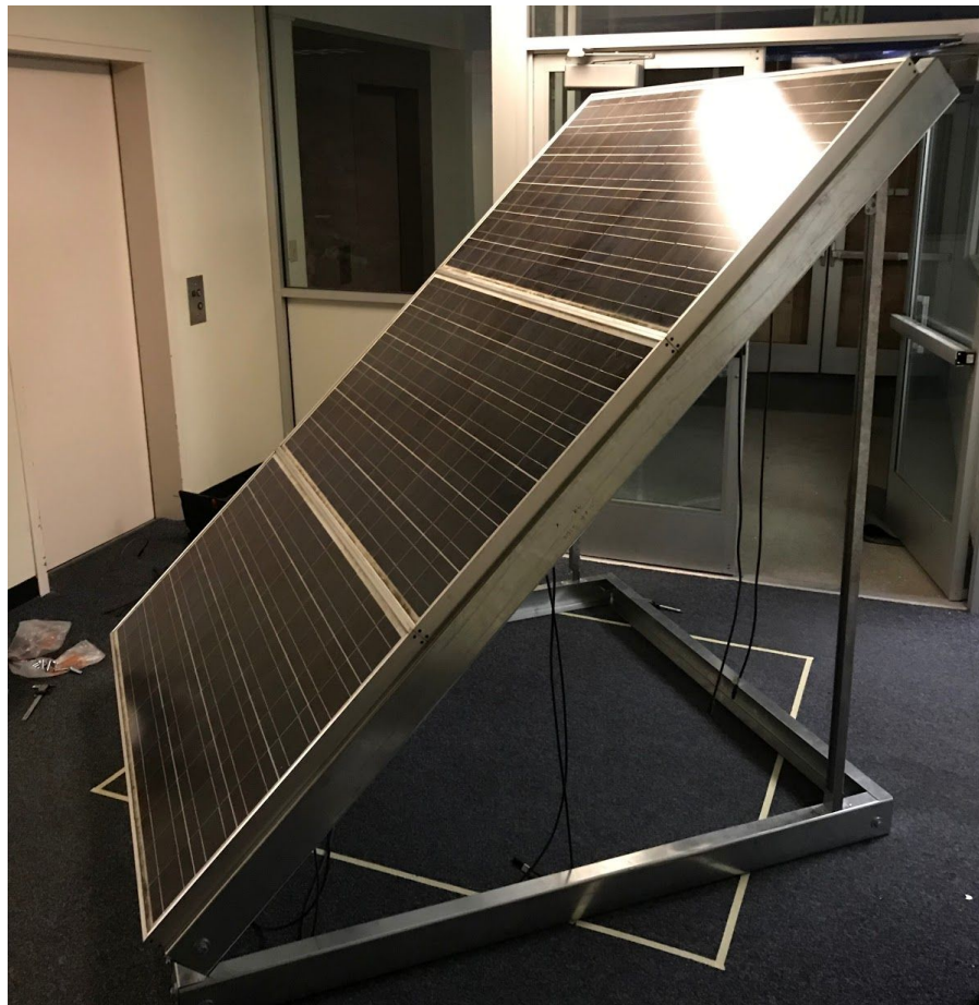
Figure 54. Fully assembled small-scale solar canopy.
