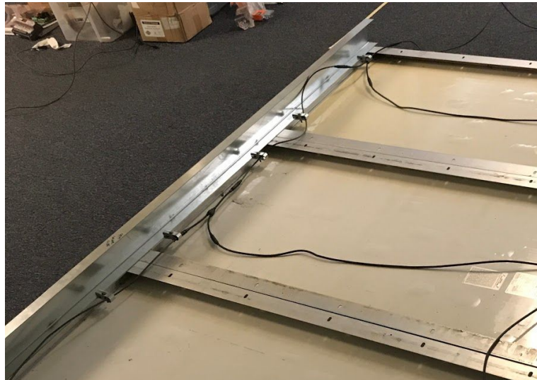
Figure 7. Back of array showing gator clamp positioning.
