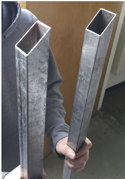
Figure 52. Square tubing cut at 45 degrees.
