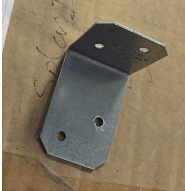
Figure 51. Bracket connecting square tubing to solar frame and base frame before modification.
