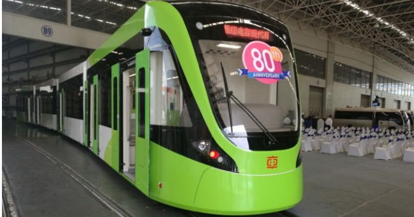
Figure 14: Light Rail system in China powered completely by supercapacitor cells.
