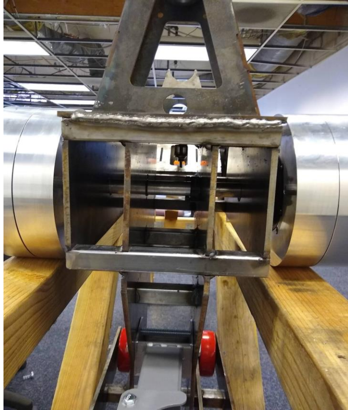
Figure 9: Location of Axle and Collars in the Drive Bogie
