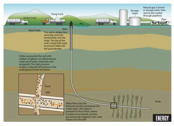
■ Fig. 13.2 Fracking procedure (From Kaufmann and Cleveland 2016)
