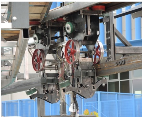
Figure 6. 2015 Full Scale Prototype. Motorized bogie and guideway section demonstrating switching ability at Maker Faire
