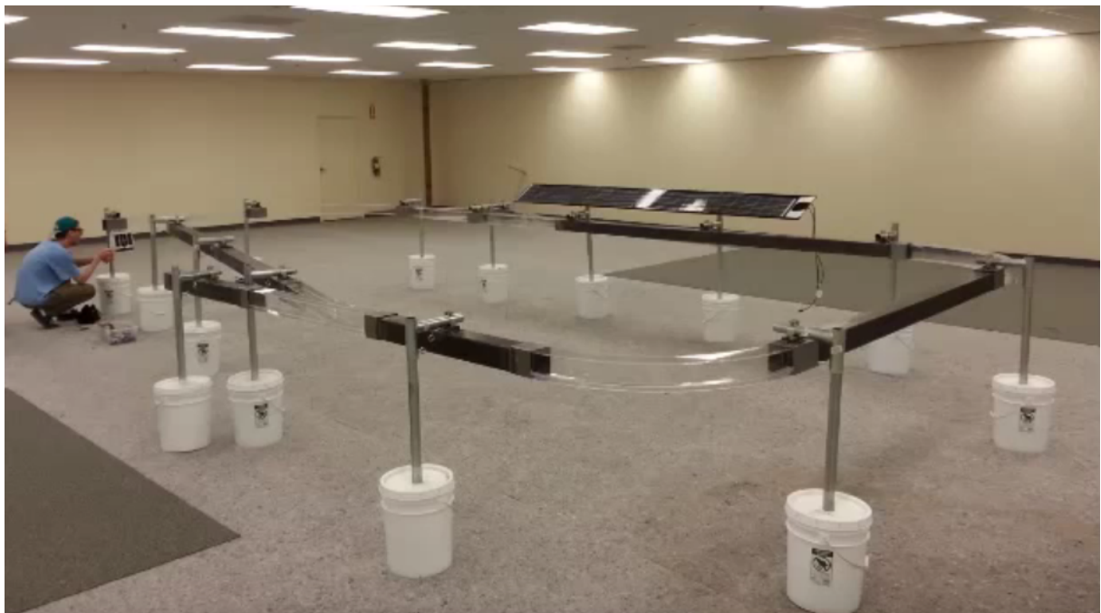
Figure 2. 2013 Scale model. 1/12th scale model of a solar powered automated transit system
