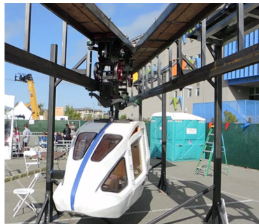
Figure 6. 2015 Full Scale Prototype. Motorized bogie and guideway section demonstrating switching ability at Maker Faire
