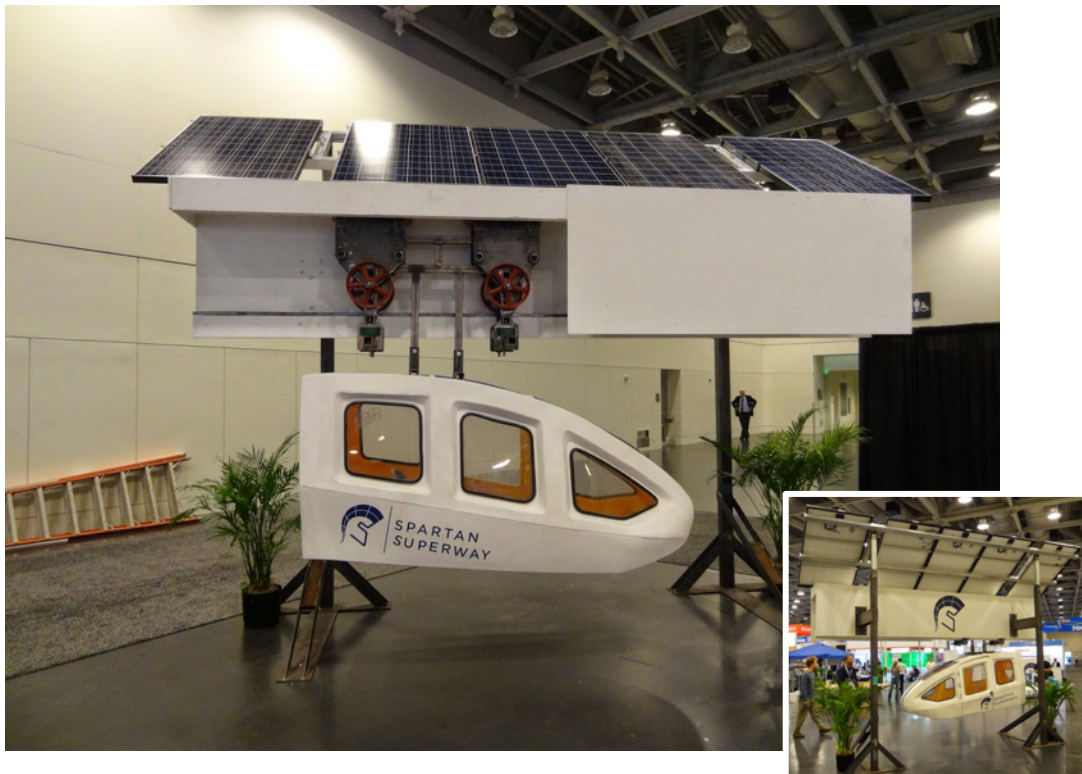
Figure 4. 2014 Full Scale. Guideway and movable bogie at Intersolar 2014 (front and back views)
