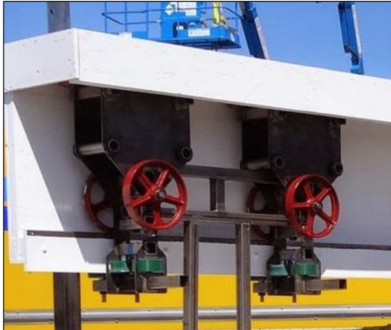
Figure 4 – Close-up of the Bogie on the Guideway system on the prototype
