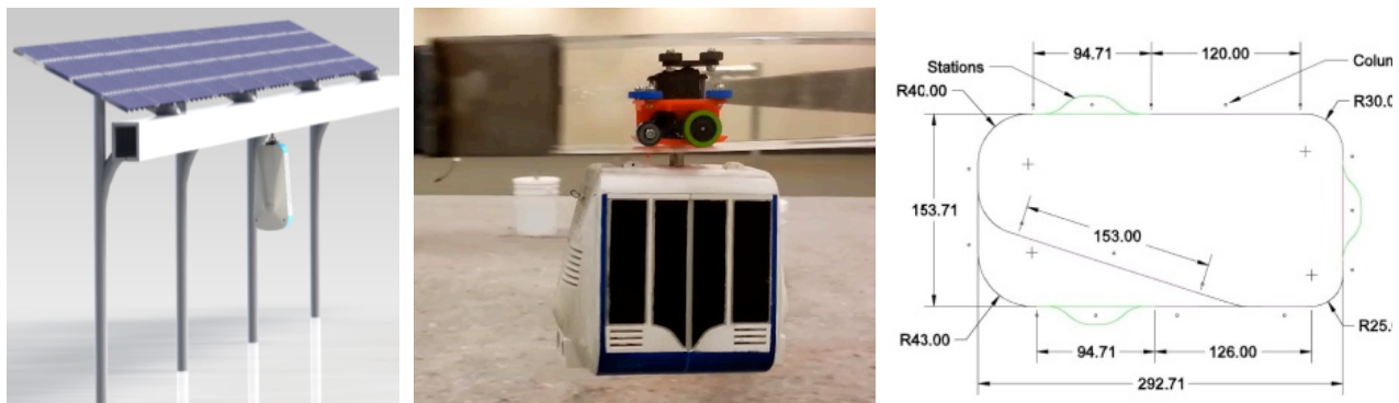
Figure 1. Accomplishments from year 1 (2012-2013) of the Spartan Superway Project. At the left, a rendering of the guideway with solar panels and suspended vehicle. At center, a 1/12 th scale bogie and vehicle traversing a guideway network, the plan view of which is shown to the right.
