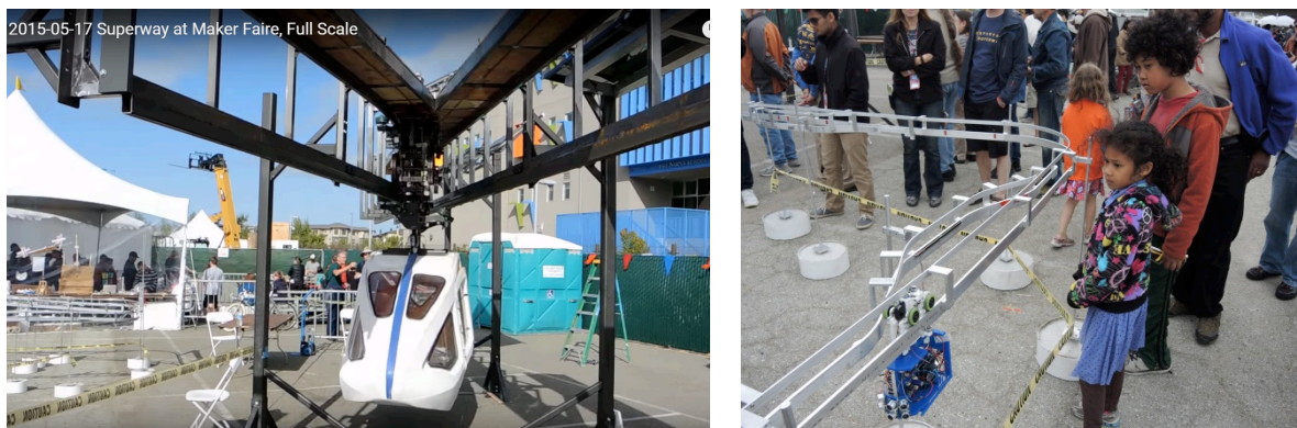
Figure 4. Spartan Superway Project at Maker Faire 2015. On the left, the full scale implementation of a 'Y' section of guideway, which supports a motorized bogie to which a mock-up vehicle cabin is suspended. On the right, the approximate 1/12 th scale model of an ATN network with autonomous vehicle in operation.
