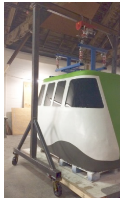
Figure 8. Accomplishments by French interns in summer 2015. On the left, the solid model of a lifting gantry. On the right, the fabricated gantry supporting the exterior cabin model.
