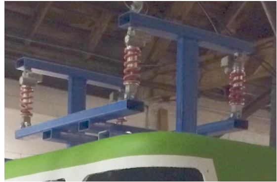
Figure 7. Accomplishments by Korean interns in summer 2015. On the left, a screenshot of the central control computer and its graphical interface. On the right, a passive suspension above the cabin model.
