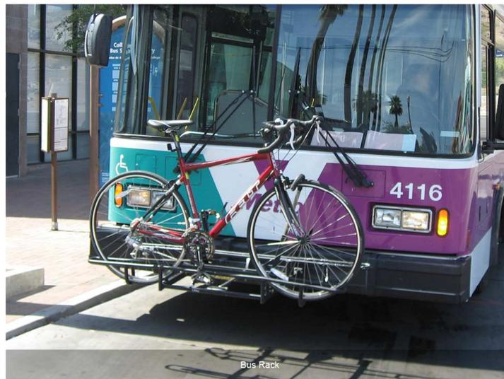
Figure 3-13: Similar form of bike storage on a public bus (cycle-works.com)
