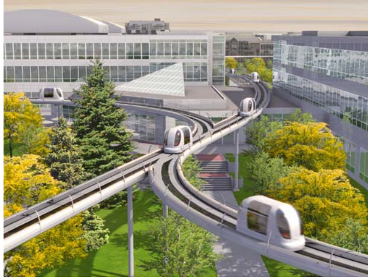
FIGURE 1.22: Example of ATN with its vehicles moving above the guideway.
