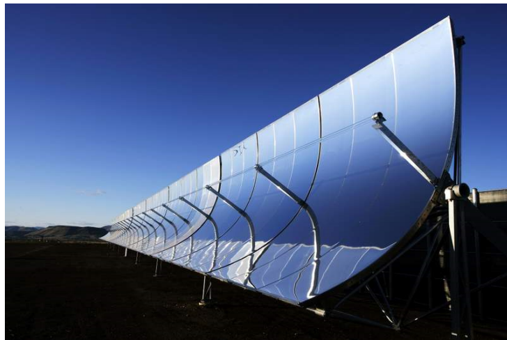
FIGURE 1.21: Parabolic Trough Concentrator. The tube is in the focus of the parabola and contains heat transfer fluid.
