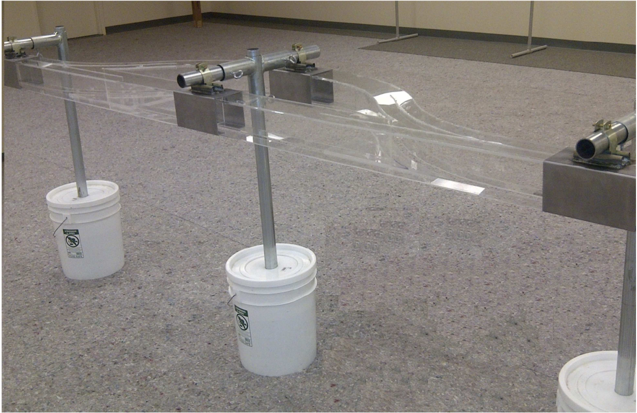
Figure 139: Acrylic Station Guide Way. This acrylic guide way was created from acrylic sheets of various thicknesses and assembled with acrylic glue, plywood moldings, and clamps.
