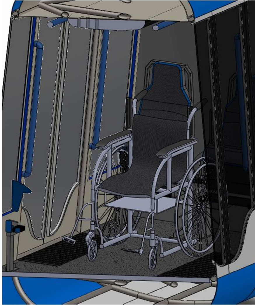
Figure 56. Angled cross section showing that there is ample room for wheelchair and follows ADA regulations
