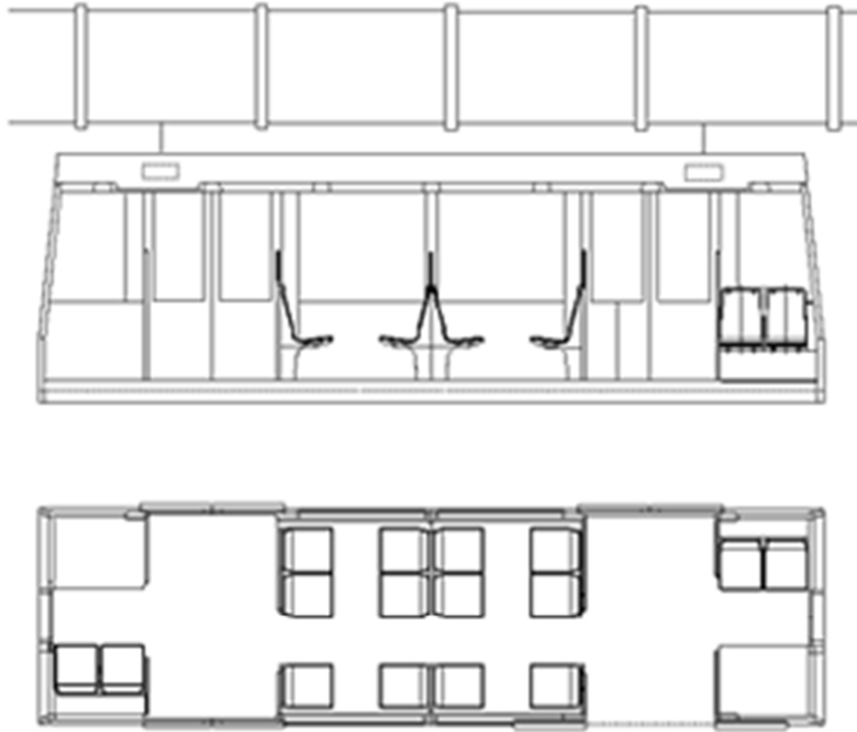
Figure 5: The H-bahn cabin features 16 seats which can accommodate multiple sized parties and the spacious layout allows for standing passengers. (H-Bahn 21)
