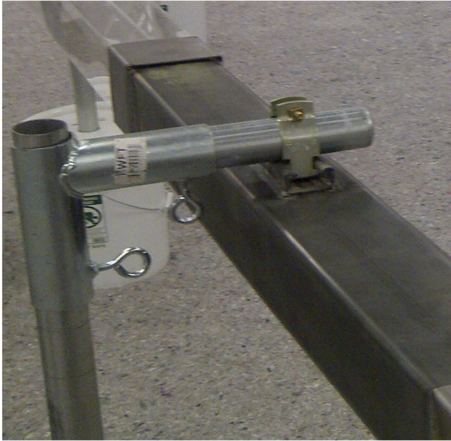
Figure 141. Example of an L shaped canopy fitting with U bracket. The supporting arm protrudes from the L shaped canopy fitting, and holds up the guide way via the U bracket.
