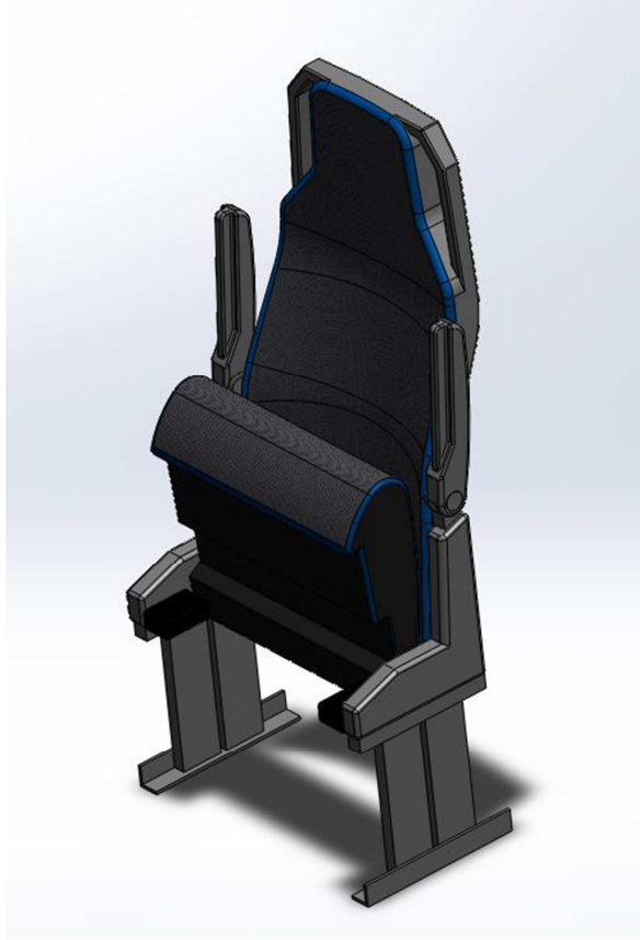
Figure 49. Neutral position of seat. Passengers will fold down the seat bottom to be seated.
