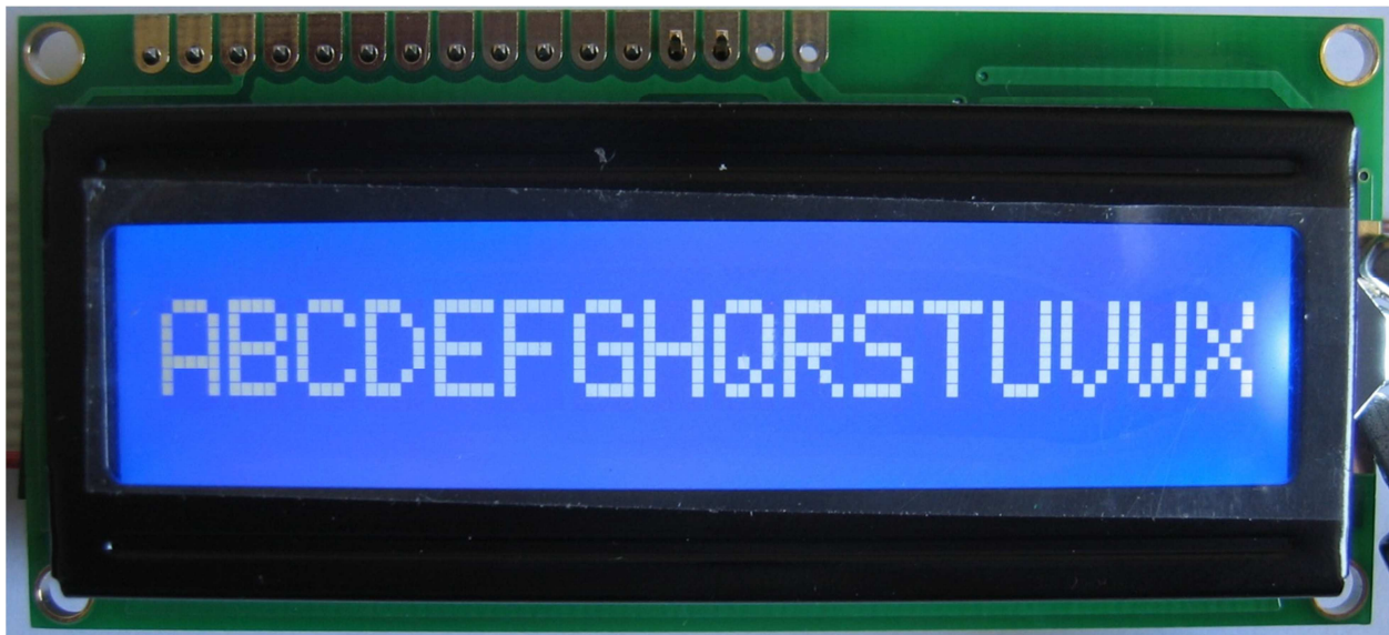
Figure 120. Actual HD44780 LCD Display (16x1 HD44780 Blue LCD, 2013)
