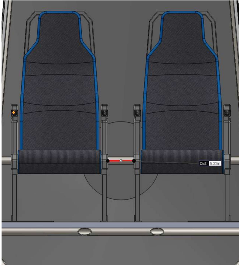
Figure 48. Space between seats allow for bicycle wheels to fit
