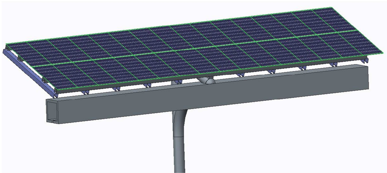
Figure 94: Frame fits two rows of panels to double the energy output
