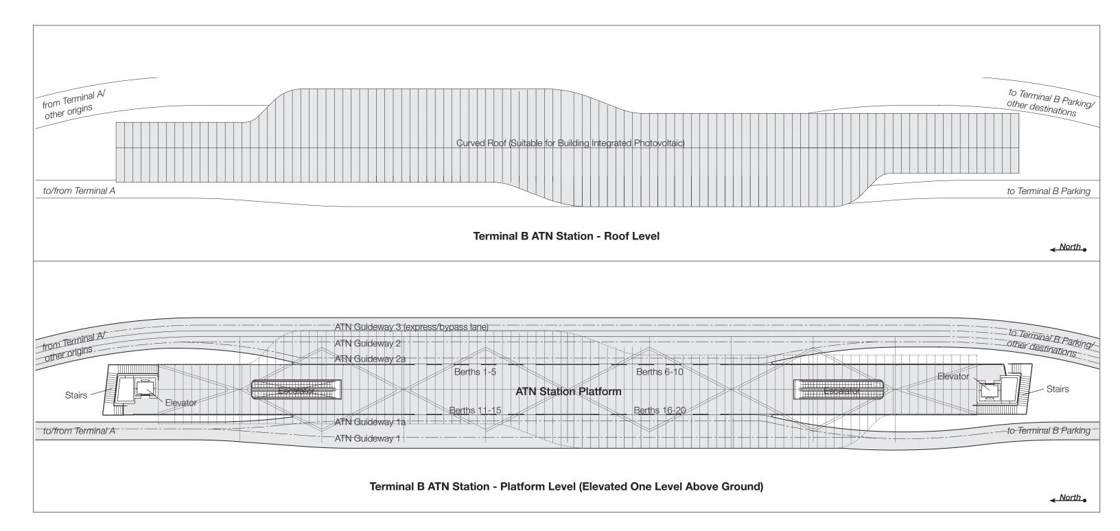
Figure 8 Terminal B ATN Station Conceptual Illustration Plan View - Roof Level and Platform Level
