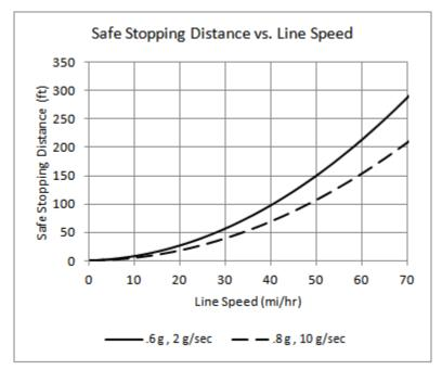
Figure 3.5-10. Stopping distance vs. line speed and deceleration rate.
