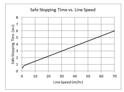
Figure 3.5-6. Safe stopping time vs. line speed.
