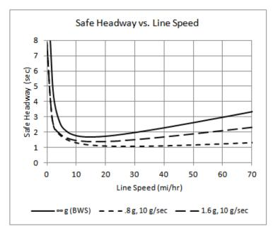
Figure 3.5-14. Headway margin within a stream of vehicles.
