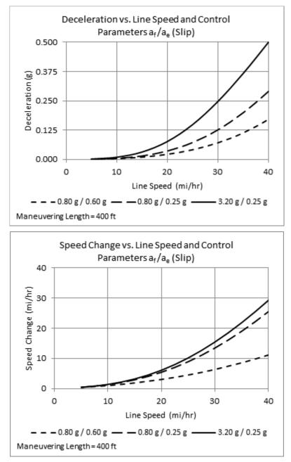
Figure 3.5-32. Minimum vehicle slip values (400-foot maneuvering length).
