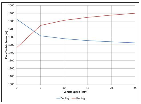
Figure 3.7-6. HVAC power requirements vs. vehicle/wind speed.
