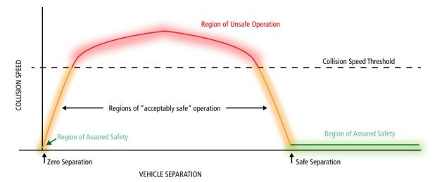
Figure 3.5-40. Collision velocity vs. separation distance revisited.
