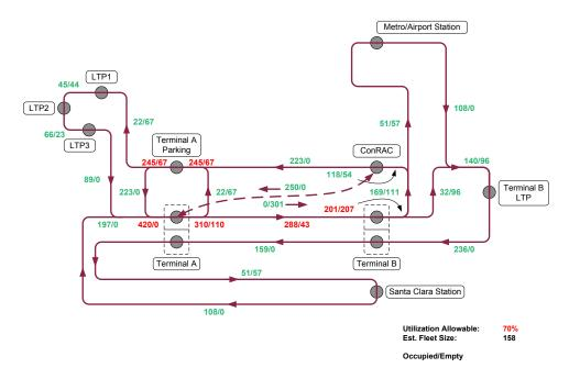
Figure 3.3-13. Alternate notional configuration + Magic Link (2030 peak hour asymmetric demand).
