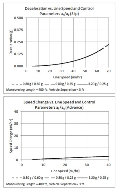
Figure 3.5-39. Minimum vehicle slip values: platoon operation.
