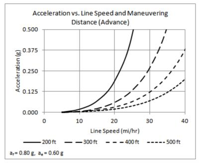
Figure 3.5-26. Minimum maneuvering acceleration (single advance).
