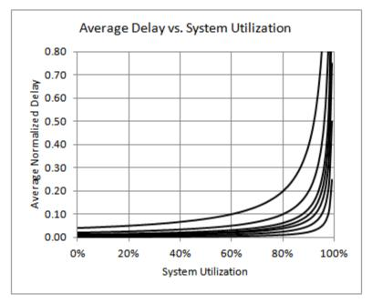
Figure 3.5-42. Average delay vs. utilization rate.
