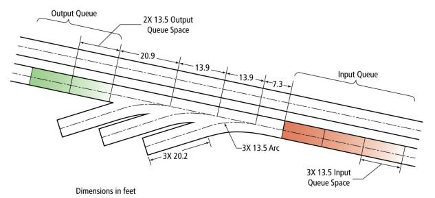
Figure 3.6-1. Angled-berth station geometry.
