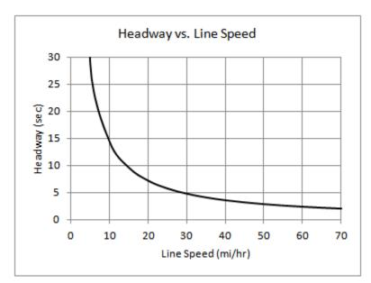
Figure 3.5-3. Time interval between vehicles vs. line speed at constant 200 ft. separation.
