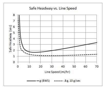
Figure 3.5-13. Safe headway vs. line speed and failure deceleration rate.
