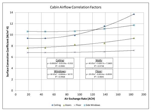
Figure 3.7-2. Convection coefficient/interior airflow correlation factors.
