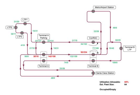
Figure 3.3-11. Alternate notional configuration (2010 peak hour asymmetric demand).
