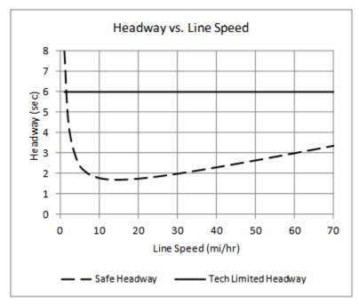
Figure 3.5-9. Comparison of safe and typical current headway.
