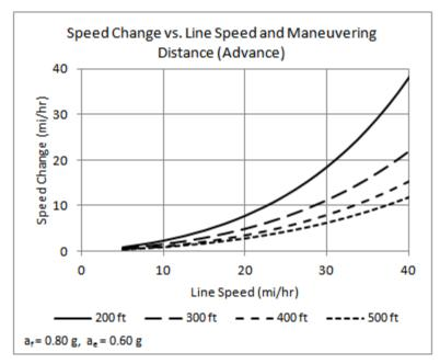
Figure 3.5-27. Minimum maneuvering speed change (single advance).
