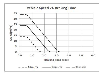
Figure 3.5-4. Vehicle speed vs. time during emergency stop.
