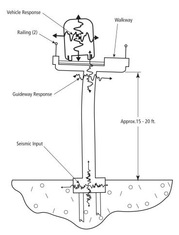
Figure 3.8-1. Seismic response of vehicle/guideway system.
