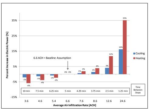
Figure 3.7-7. HVAC power vs. cabin air exchange.
