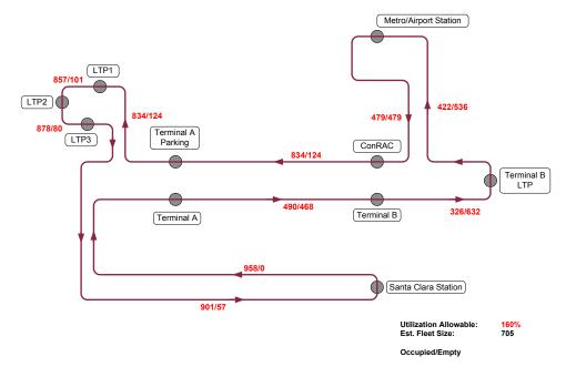
Figure 3.3-10. Notional configuration (2030 peak hour asymmetric demand).
