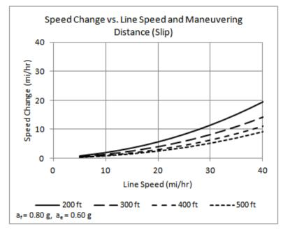
Figure 3.5-29. Minimum maneuvering speed change (single slip).
