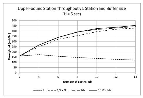
Figure 3.6-4. Upper-bound throughput vs. station and buffer size (6-second headway).
