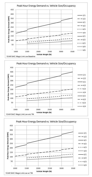
Figure 3.10-27. Peak hour energy demand vs. vehicle size/occupancy and thermal management.
