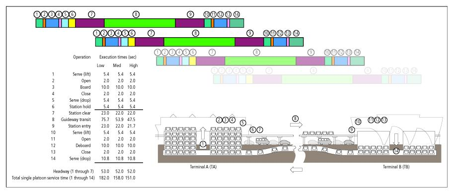
Figure 3.10-25. Magic Link subnetwork trip times and headway.
