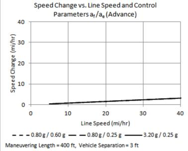
Figure 3.5-38. Minimum vehicle advance values: platoon operations.
