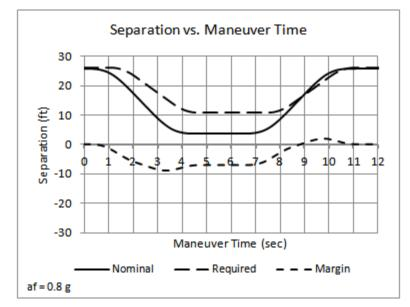
Figure 3.5-20. Separation margin (0.8 g failure deceleration).
