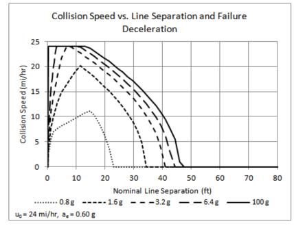
Figure 3.5-16. Collision speed vs. separation distance vs. failure deceleration rate.
