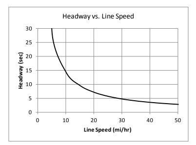
By including the fact that *safe* separation distance is *not* constant relative to line speed, a curve for safe *headway* relative to line speed can now be generated. This is shown below in Figure 3.5-8.
