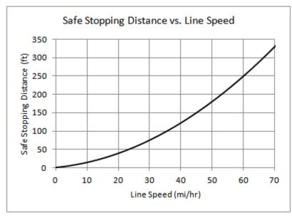
Figure 3.5-7. Safe stopping distance vs. line speed.
