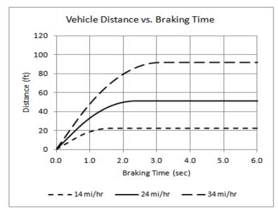
Figure 3.5-5. Vehicle braking distance vs. time during emergency stop.
