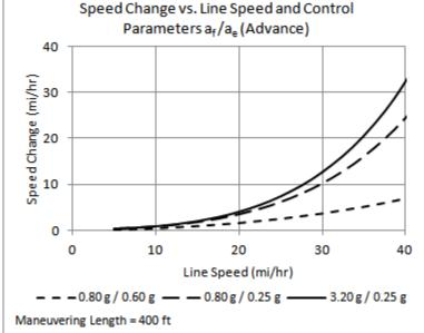
Figure 3.5-33. Minimum vehicle 50/50 advance values (400-foot maneuvering length).
