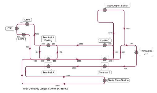
Figure 3.3-3. Alternate notional configuration.
