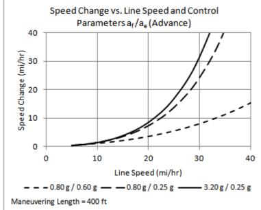
Figure 3.5-31. Minimum vehicle advance values (400-foot maneuvering length).
