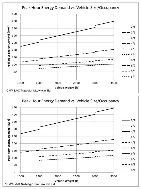
Figure 3.10-29. Peak hour energy demand: effect of Magic Link Low operation.
