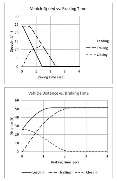
Figure 3.5-12. Vehicle pair speed and separation: emergency stop.
