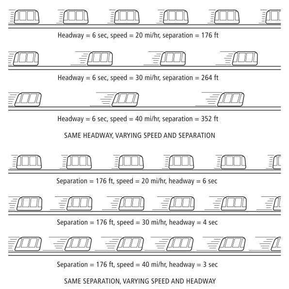
Figure 3.5-2. Relationship between headway, speed, and separation distance.
