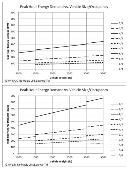
Figure 3.10-32. Peak hour energy demand: propulsion type comparison.
