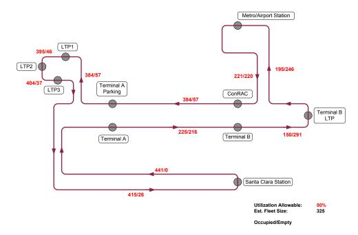
Figure 3.3-9. Notional configuration (2010 peak hour asymmetric demand).
