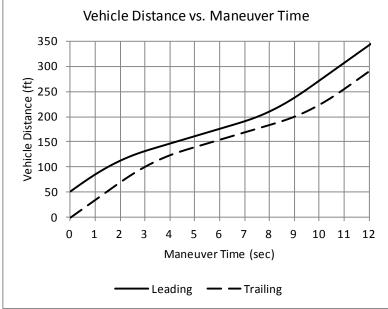
Figure 3.5-18. Two vehicles negotiating a curve.
