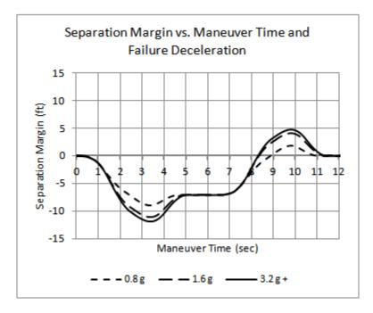
Figure 3.5-21. Separation margin vs. failure deceleration rate.
