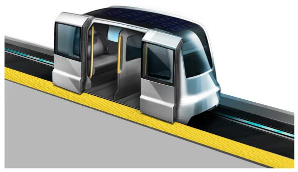
Figure 3.10-18. Non-ADA-compliant vehicle.
