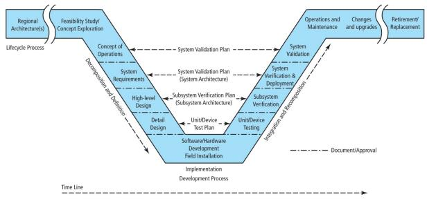
Figure 4.1-1. FHWA systems engineering process.
