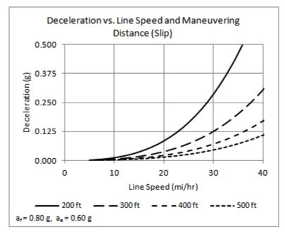
Figure 3.5-28. Minimum maneuvering deceleration (single slip).
