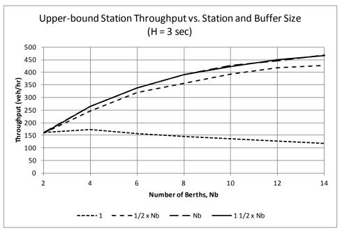
Figure 3.6-5. Upper-bound throughput vs. station and buffer size (3-second headway).
