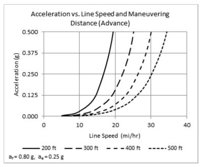
Figure 3.5-30. Minimum maneuvering acceleration (single advance,  $a_e = 0.25$  g).
