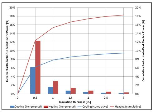
Figure 3.7-5. Potential HVAC power savings from cabin insulation.
