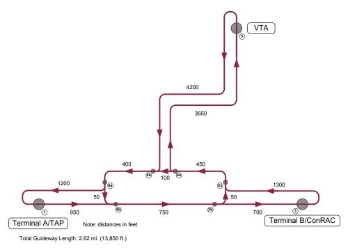
Figure 3.3-15. Routing study configuration topology.
