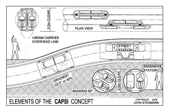
CAPSI's novel solution is to provide two rails, one below and one overhead, and to give the capsule four wheels, two below and two above. John Stegman holds a provisional patent on this design.
