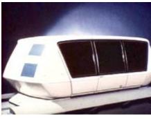
arly 1960's, a group at General Motors Research Laboratories had been working on ground-effects machines for the Army. These were air-suspended vehicles that could run on a variety of surfaces, but with such low power on paved roads that air suspension appeared applicable to transit. Since an air-suspended vehicle made no direct contact with the roadway, a new type of motor was required that did not use wheels for traction. The
