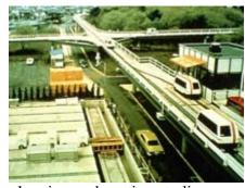
**CVS**. The Computer-Controlled Vehicle System (CVS) is a one-second-headway, 2000-lb, four-passenger-vehicle PRT system developed in Japan beginning in 1968. Scale models were built, a 1000vehicle network was simulated, and a full-scale test facility began operating in 1972 in a suburb of Tokyo with 4.8 km of guideway and 60 vehicles. Extensive
