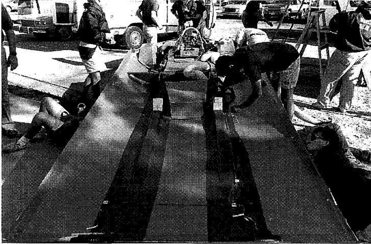
Like Pomona and George Washington, sixth place Maryland used a chassis with central carbon beams and cross bulkheads.
