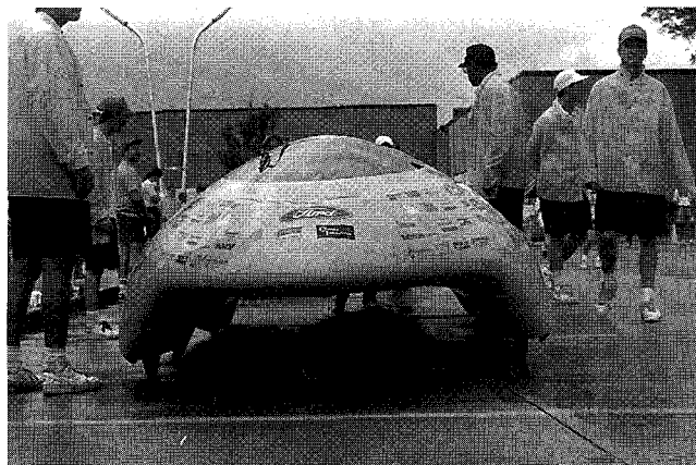
Front and rear views of the first place University of Michigan "Maize & Blue." The catamaran type chassis gives better solar array exposure in morning or afternoon sunlight when the solar angle is less than 90°.
