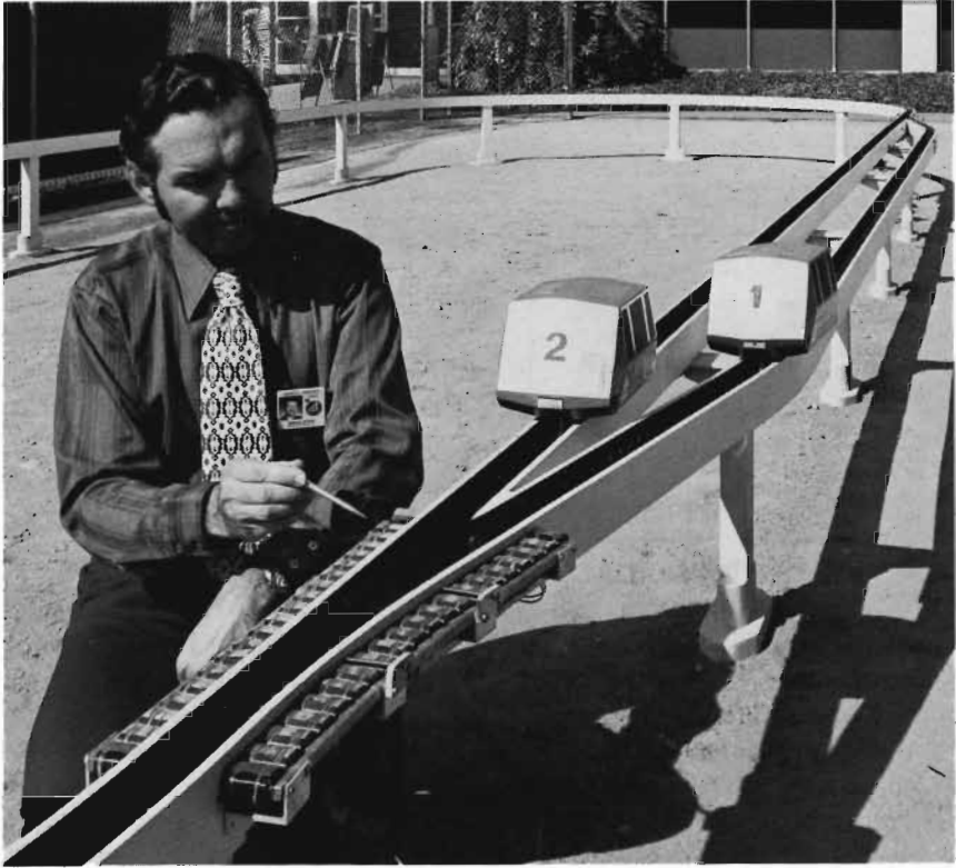
Fig. B-6. Electromagnetic Switch Installation
