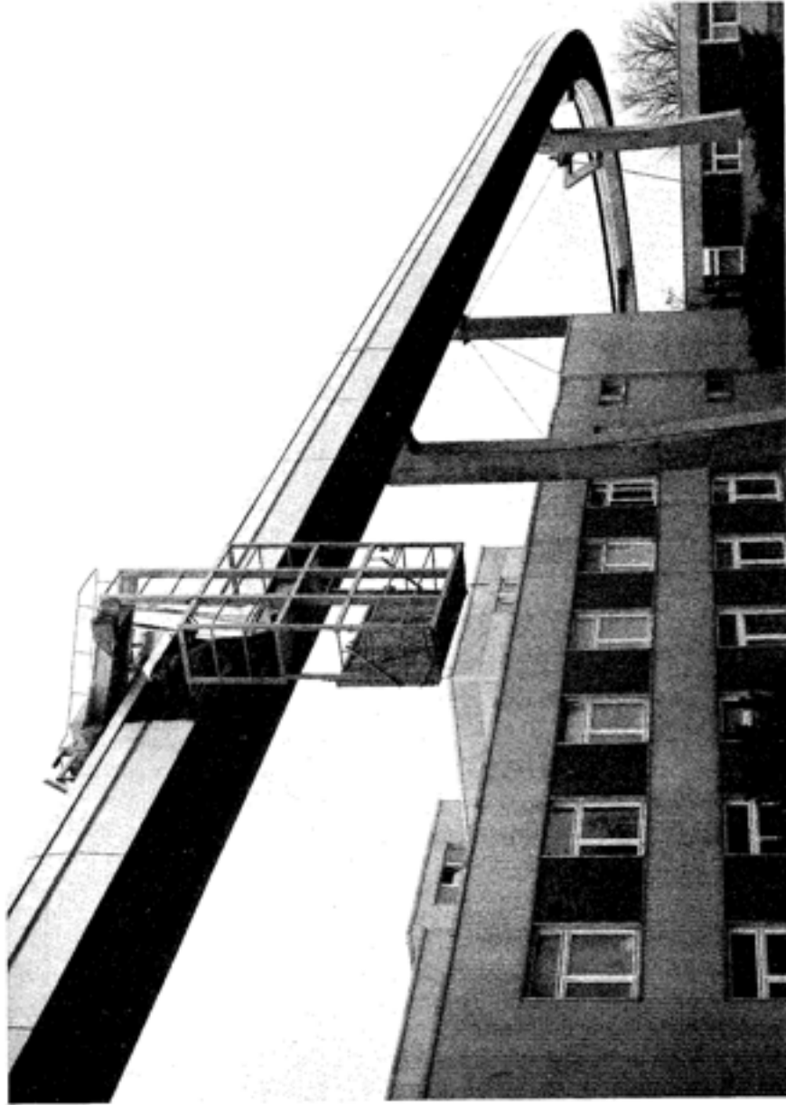
Figure 9-4. Service Vehicle in Operation on the Side of the Guideway of The Cabinlift System—at the Ziegenhain The photo is of F. v. L. West Germany. Courtesy of DEAFAC, 1988.
