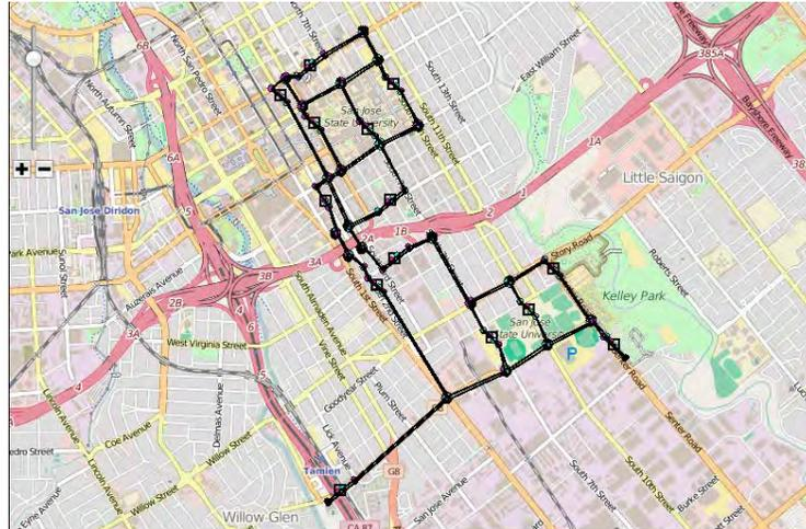
**Figure 5: Proposed guideway placement for the Superway in San José.** The layout of guideways and stations connects the south and north parts of San José State University and the Tamien Caltrain/Light Rail stations. The total length of the guideway is about 14 km. A canopy of monocrystalline PV approximately two to three meters wide above the guideway would be sufficient to power the system. (Route map made using RouteTime software from Jpods (<http://www.jpods.com/tools>))
