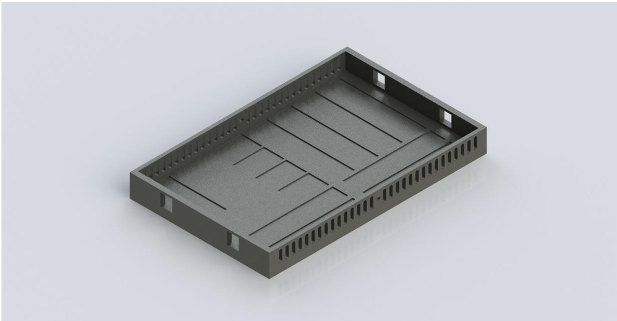
*Figure 22: Full-size Power Module. Dimensions: 72 in. x 42 in. x 3 in.*
