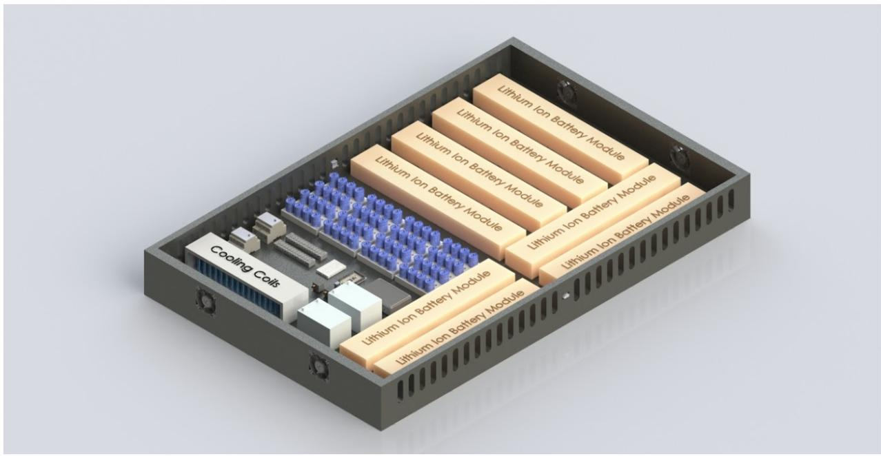
*Figure 21: Full-size Power Module with all-electric components.*
