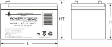
Tolerances are +/- 0.04 in. (+/- 1mm) and +/- 0.08 in. (+/- 2mm) for height dimensions. All data subject to change without notice.
