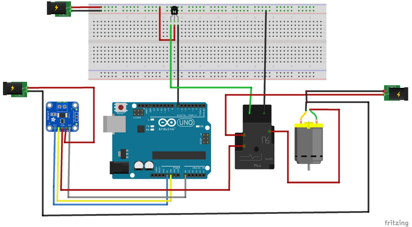
Figure 11: Electrical Schematic of the 2019-2020 Power Module.
