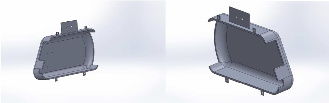
Figure 2-18: The cabin will be 3D printed as two half shells to allow easy assembly and allow easy access when mounting circuit components.
