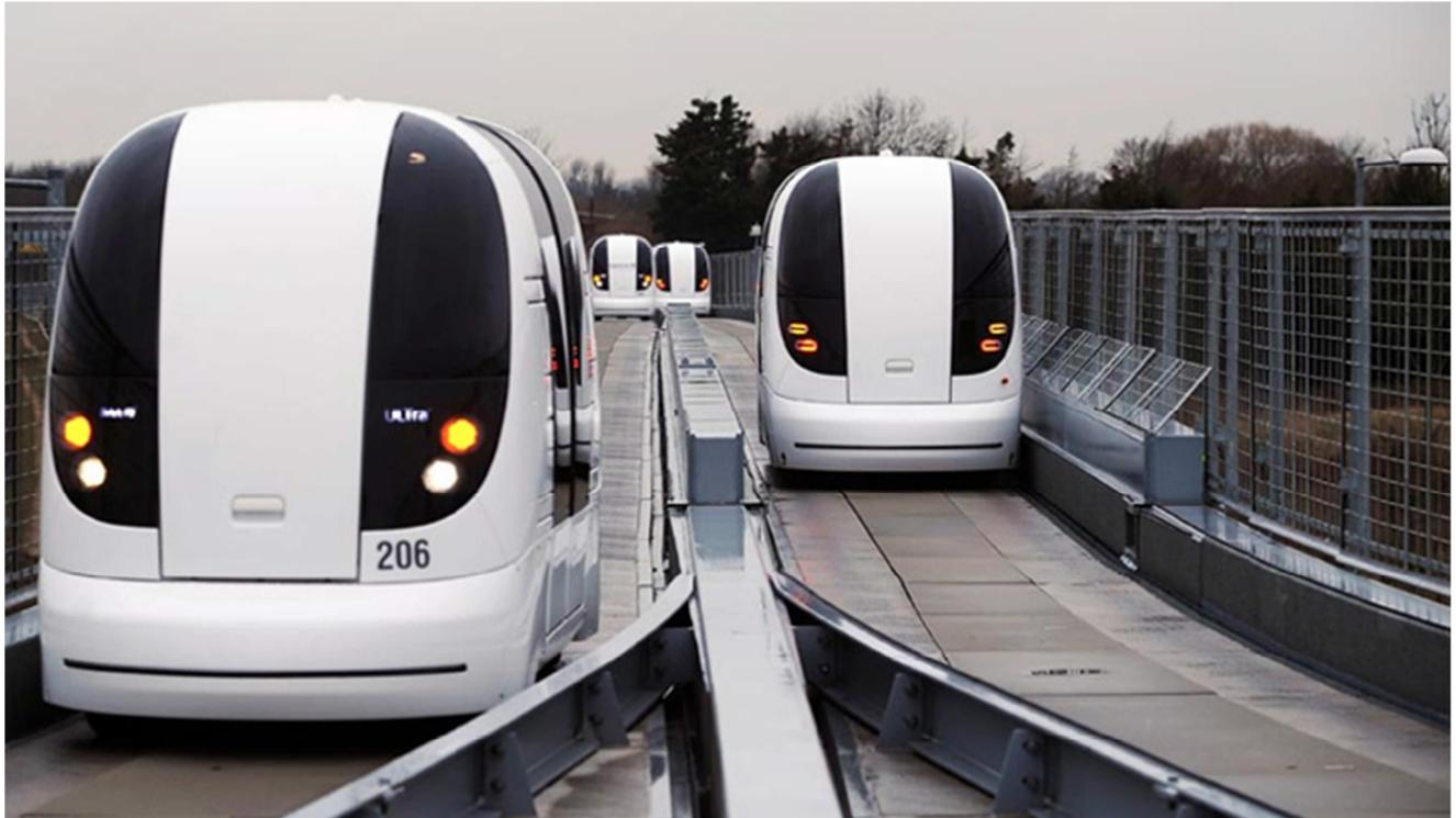
*Figure 2-20: The Ultra PRT is fully operational in Heathrow London. This system uses battery-powered pods to travel on a 3.8 km track (ULTra, 2014).*
