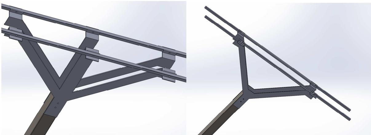
Figure 4-15: Initial Mount Design for Solar Panels. The design on the left allows for a more stable base. Both designs have ¼ inch aluminum rails that will be secured by screws. The rails will be where the solar panels will be attached.
