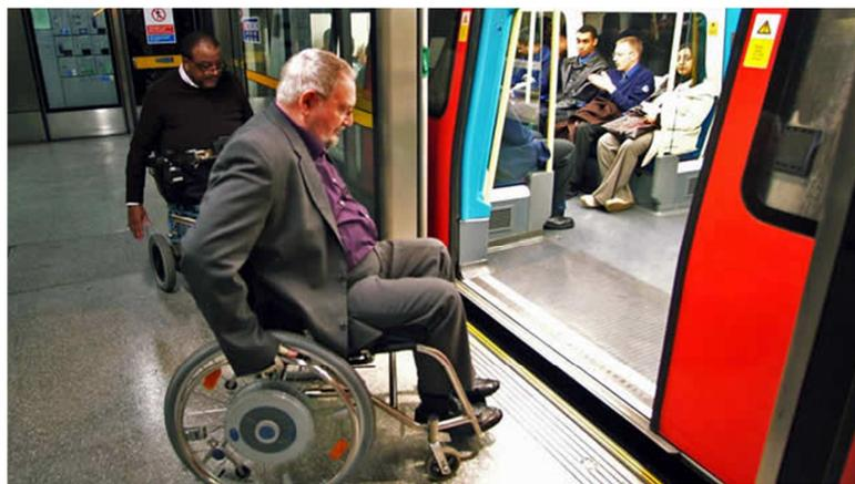
Figure 3-41 The position of the cabin and station platform must be level in order to ensure passenger safety and convenience
