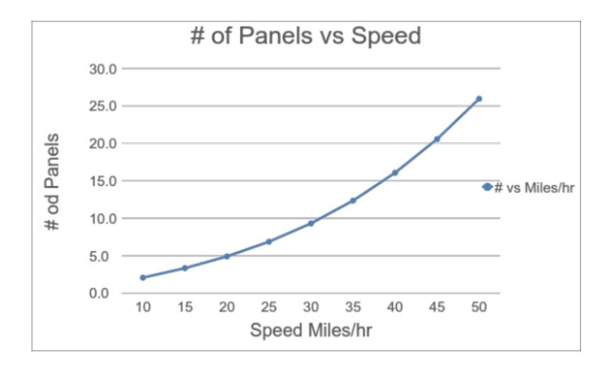
The above graph shows the number of panels required to move the vehicle at constant velocity
