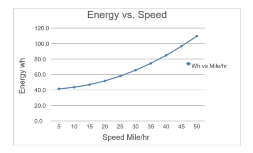
The above graph shows the amount of energy required to move the vehicle at constant velocity
