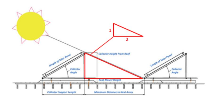
Using a 2 to 1 spacing to height ratio, the maximum number of panels that can be included in a 1 km length is 1,234 panels. This number of panels can produce 2,308 kWh of DC energy per day on average.
