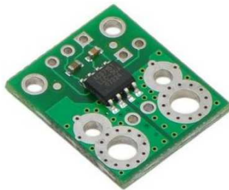
Figure 5: ACS714 Current Sensor Board
