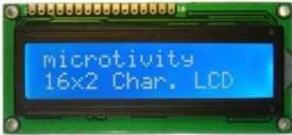
Figure-26: LCD Module with specifications
