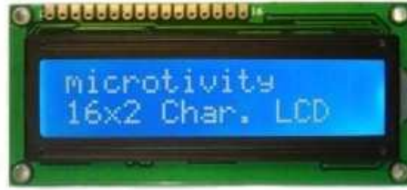
Figure 7: Microtivity Arduino compatible 16x2 Character LCD module
