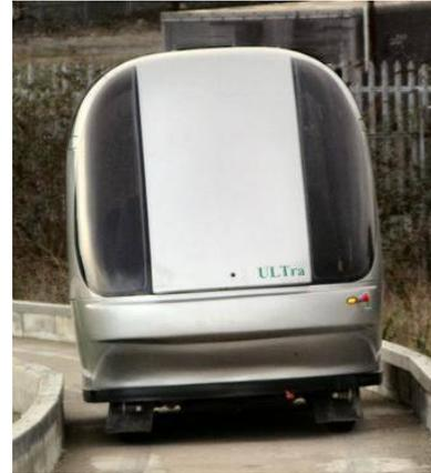
**Figure A-4 - ULTra Vehicle On Surface Guideway**
