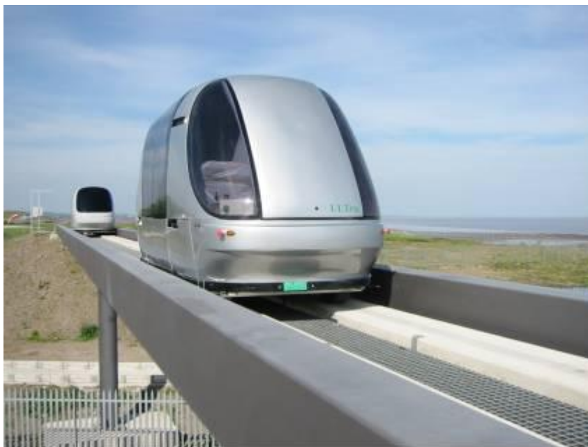
Figure 1 ULTra Vehicles on the Cardiff test track
