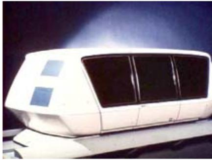
Research Laboratories had been working on ground-effects machines for the Army. These were air-suspended vehicles that could run on a variety of surfaces, but with such low power on paved roads that air suspension appeared applicable to transit. Since an air-suspended vehicle made no direct contact with the roadway, a new type of motor was required that did not use wheels for traction. The
